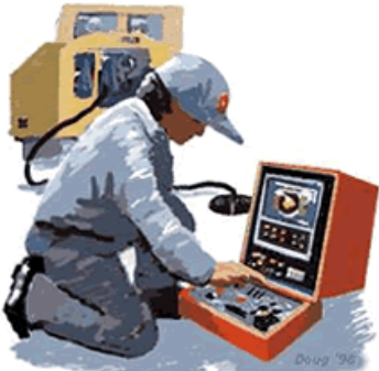
One of the ways to identify illicit connections is by inspecting storm drain system using video equipment (Source: Drain Patrol, no date)
